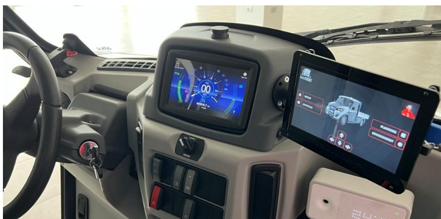
Figure 5: HMI set-up including a dedicated monitor, on the right, for driver assistance
